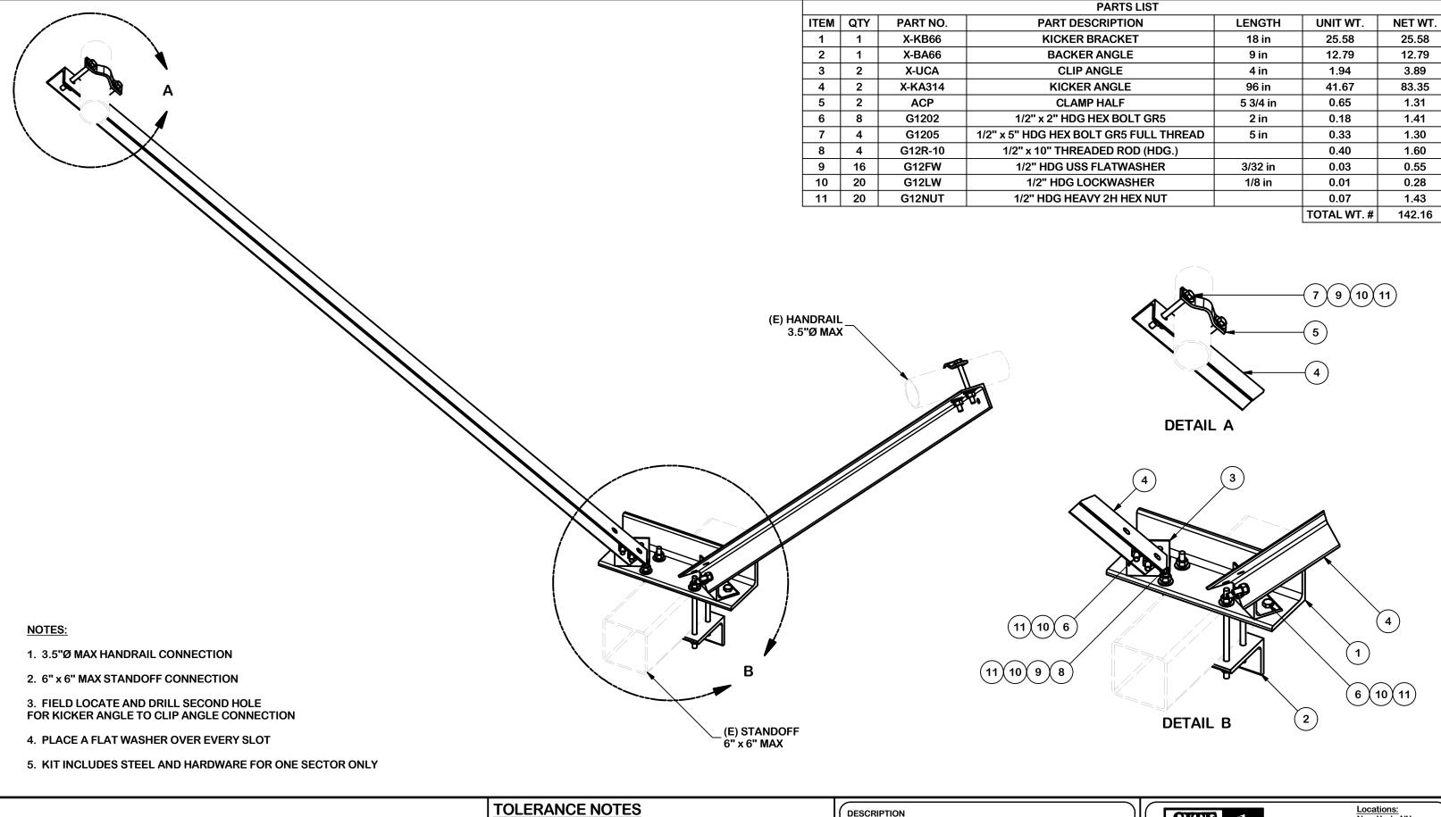
TOLERANCES ON DIMENSIONS, UNLESS OTHERWISE NOTED ARE: SAWED, SHEARED AND GAS CUT EDGES ( $\pm\,0.030$ ") DRILLED AND GAS CUT HOLES (± 0.030") - NO CONING OF HOLES LASER CUT EDGES AND HOLES (± 0.010") - NO CONING OF HOLES BENDS ARE ± 1/2 DEGREE
